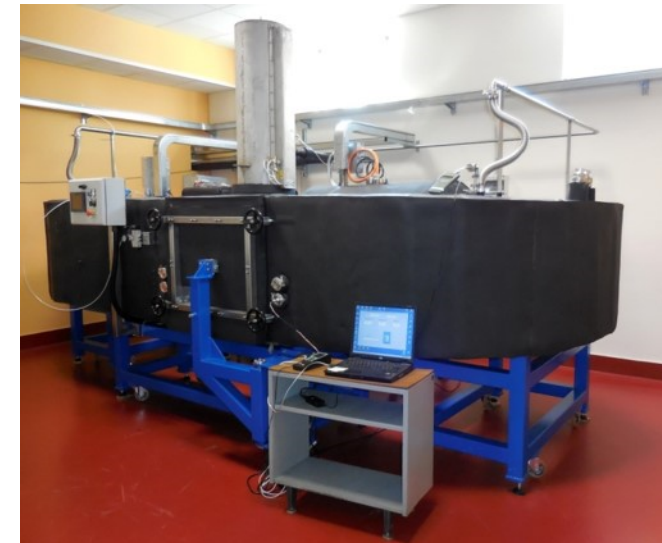
Wind tunnel EDDIE for the characterization of temperature sensors. Source: www.inrim.eu
