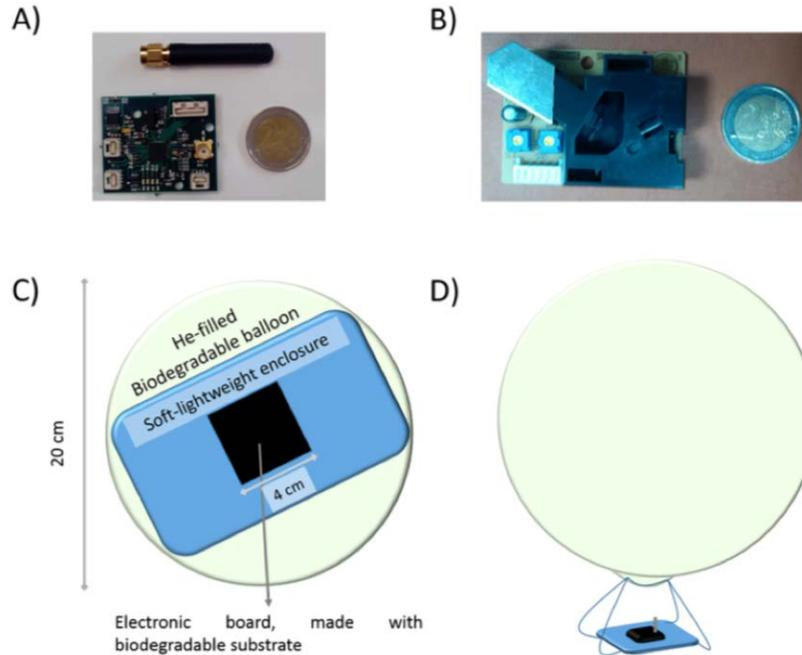
Figure 1 A) Early prototype electronic board. B) Example of the OPC (Rorato et al. *Wireless Sensor Network* 2013). Possible probe designs: C) ultra-lightweight model in which the electronics are comfortably placed into the He-inflated balloon and D) advanced radiosonde where the electronics hang from the balloon.
